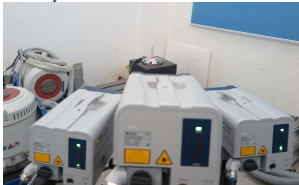
Figure 10. 3D-SLDV modal test
