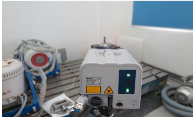
Figure 8. 1D-SLDV modal test
